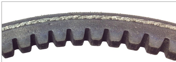
Figure 2 The sidewall of used notched V-belt
