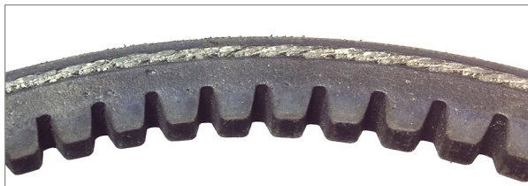
Figure 2 The sidewall of used notched V-belt
